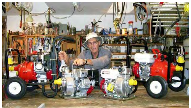
The red foam pumps are Gorman Rupp's model OTC-5265HC. The smaller aluminum draught pumps are Honda's model WH15XK1C1
